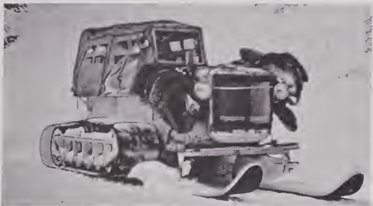
FIGURE 4. Tucker Sno-Cat (M-7 Snow Tractor) used by Army Air Forces for rescue and ground reconnaissance missions but later discarded.
